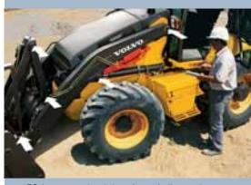
50-hour greasing intervals, and all greasing points are accessible from the ground level.
